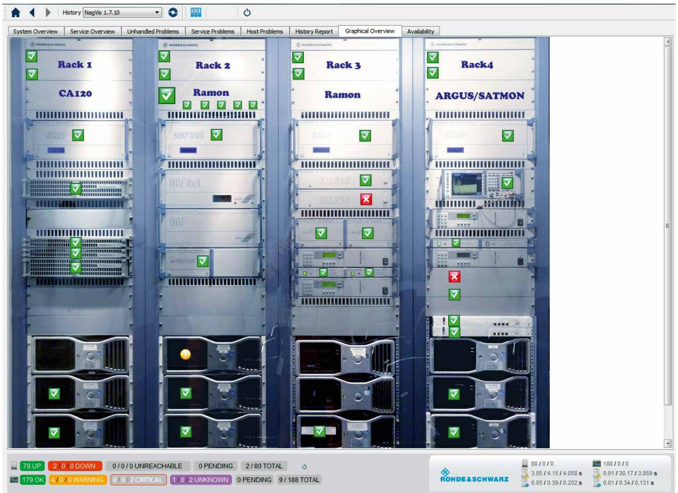
Fig. 3: System status overview. Realistic hardware views can be integrated into the software to give users fast visual orientation on system status.
