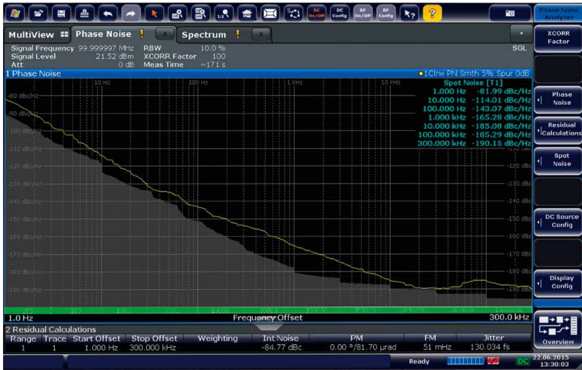
Fig. 2: Trace of a high-end OCXO with -190 dBc (1 Hz) phase noise at a frequency offset of 1 MHz.
