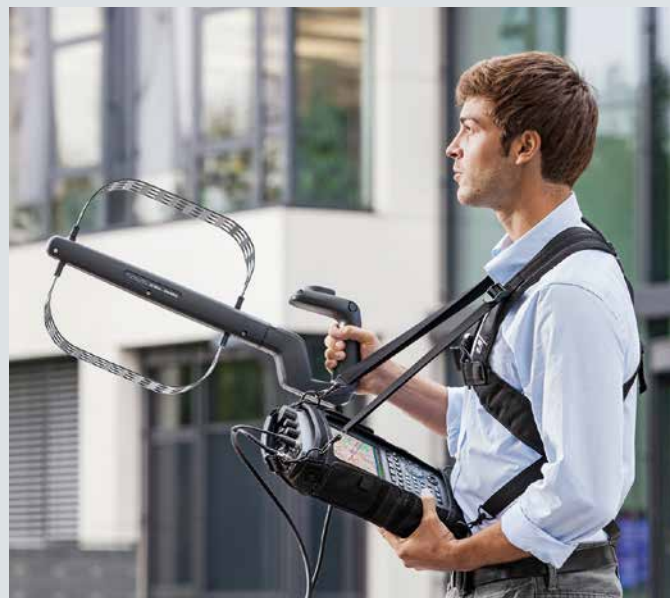
Fig. 4: Mobile measuring receivers with directional antennas help operators monitor operational networks and identify interference.
