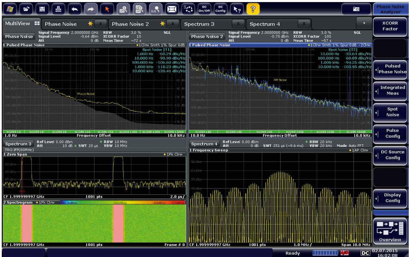
Fig. 5: Measuring a pulsed signal in the time and frequency domain with the spectrum analyzer (below) and with the phase noise analyzer (above). The upper left window shows the phase noise of the pulsed source; the upper right window displays the amplitude noise. The distance between the noise measurement traces and the gray area below represents the sensitivity improvement by cross-correlation. The segments where there is no distance between trace and gray area indicate that additional cross-correlations are required to achieve an unambiguous measurement result.
