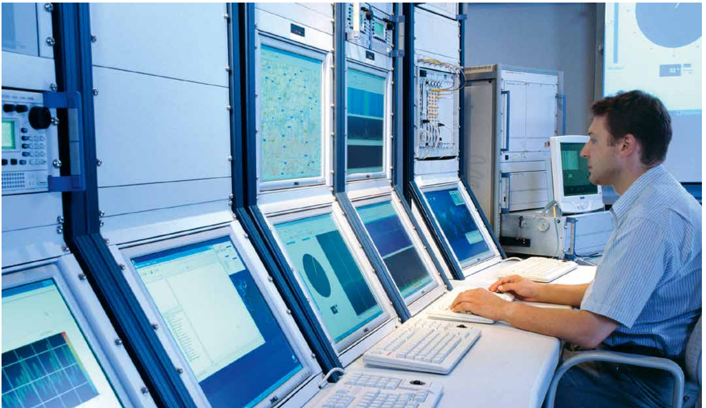
Fig. 1: The new R&S®RA-CHM system status monitoring software records the operating parameters of all components in large distributed radiomonitoring systems, compares them with nominal values and triggers alarms when target values are not met.
